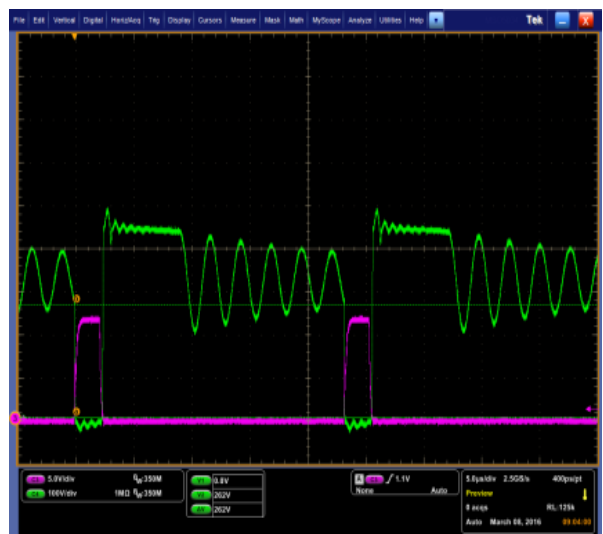
230 VAC, 6 th Valley Ch. 3 (Purple): DRV Ch. 4 (Green): Drain Voltage
