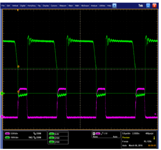
230 VAC, 1 st Valley Ch. 3 (Purple): DRV Ch. 4 (Green): Drain Voltage
