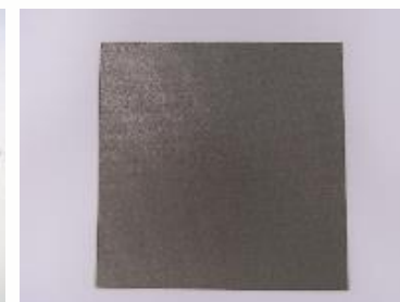
Make sheet by blending & dispersing magnetic powder in polymer
