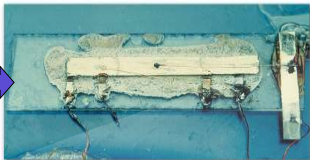
Jack Kilby's first working integrated circuit, tested on September 12, 1958,
