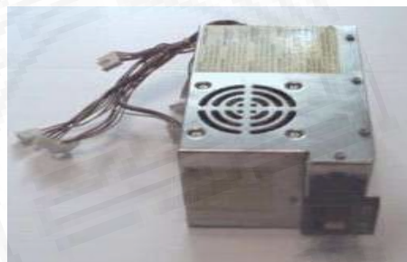
IBM PC/XT power supply 1983 : 63.5W
