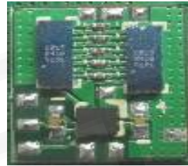
Parallel loop 2 ( 0.2nH ) 9mm*9mm
