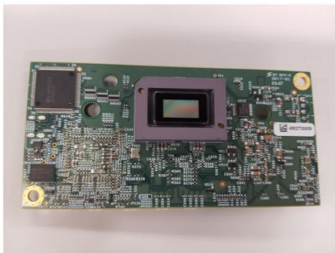
EVM Front Side with DMD mounted
